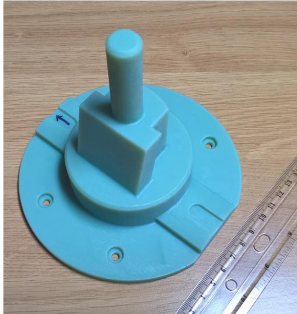
Polymer artefact: MTC modified version of open National Institute of Standards and Technology (NIST) design, 3D-printed in ABS on Stratasys Objet 1000 machine
